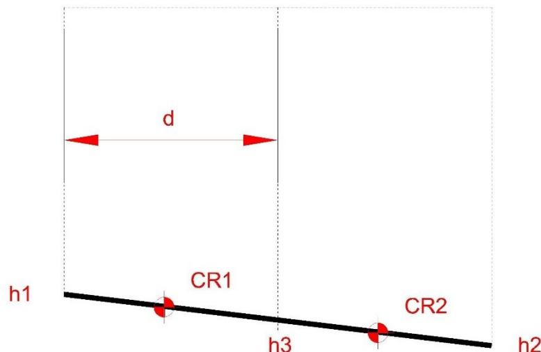
$$\begin{aligned} &\text{Para } (h1-h2) > 1,5 \text{ m} \\ &CR1 = h3 + ((h1-h3)/2) \\ &CR2 = h2 + ((h3-h2)/2) \\ &d > 6 \text{ m} \end{aligned}$$
